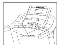
Next, stand on the foot rails and hold the metal contacts—avoid moving your hands. When your pulse is detected, your heart rate will appear on the screen. For the most accurate heart rate reading, continue to hold the contacts for about 15 seconds.
